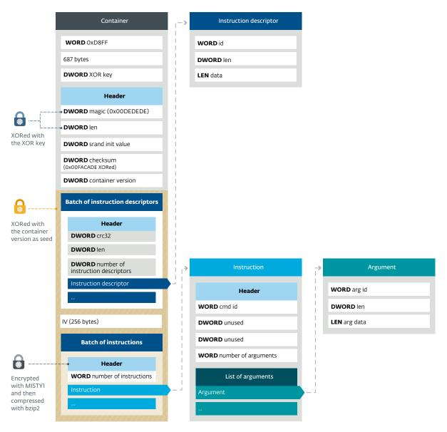
Figure 20 // Structure of the command container
